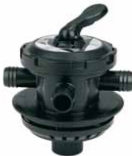
6-way multiport valve for above ground pool filters where the pressure does not exceed 1.5 bar, of maximum diameter 380 mm. Bayonet closing system.
